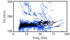
*Figure 2* An example of the SASW-like cloud of points in the f- $V_R$  domain. In this example, the blue points are filtered out while the black points are those which comply with eq. 2.
