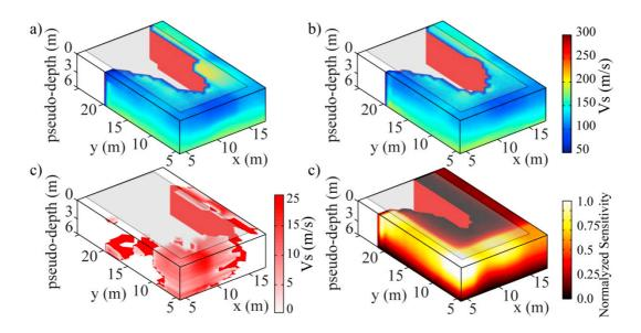
**Figure 3** Apparent  $V_s$  (a) before and (b) after the resin injection. c) Stiffening effect in term of percent increase of  $V_s$ . d) Normalized sensitivity accounting for the reliability of the results. Portions of the model for which to retrieve any result was not possible with the present sources-receivers configuration are not colored. The footprint of the building is highlighted with the gray rectangle.
