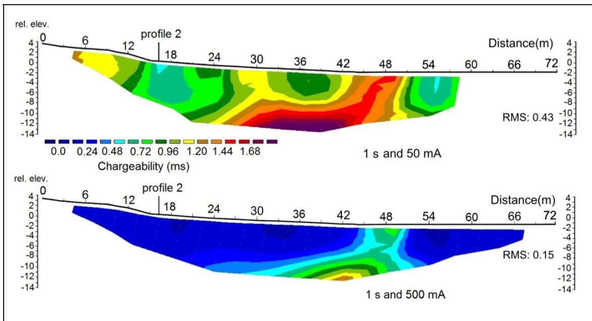
Figure 3 Chargeability model sections of profile 1. Above: section obtained at 50 mA of supplied current; below: section obtained using a supplied current of 500 mA.
