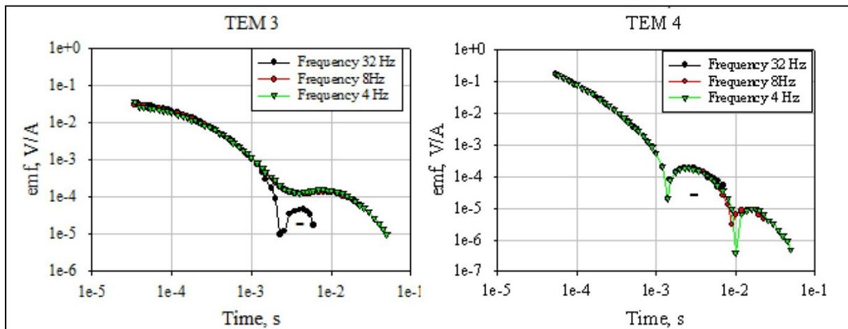
**Figure 4** Decay curves of TEM soundings 1-6 (continuous line: best-fitting 1D model).
