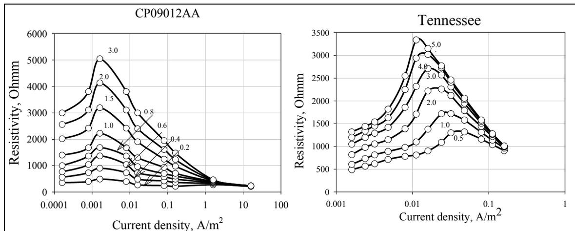
**Figure 1** Resistivity has direct relationship with current density if the latter is small and reverse relationship if current density is larger: circles: laboratory measurement data, curve: theoretical fitting data. Numbers on the curves indicate time of current flow (in seconds).
