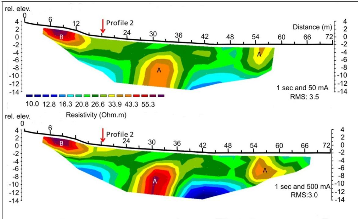
Figure 2 Resistivity model sections of Profile 1. Upper window: section obtained at 50 mA of supplied current; lower window: section obtained using a supplied current of 500 mA.
