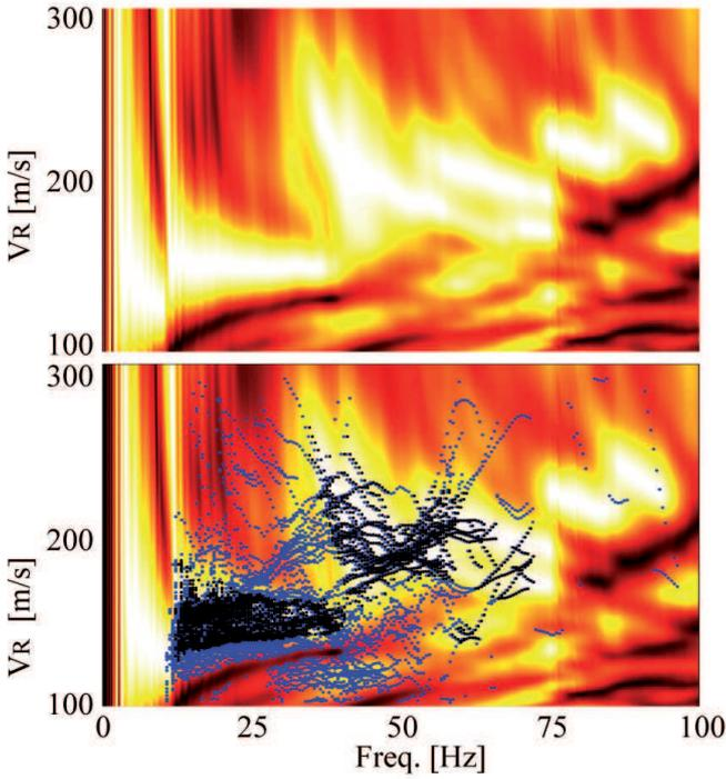
Fig. 1 – An example of the SASW-like cloud of points in the f-VR domain. In this example, the blue points are filtered out while the black points are those which comply with Eq. 2. For sake of comparison, the corresponding frequency-velocity transform is shown both clean (above) and with superimposed points (below) to show how the filtered COP adapts to the propagating modes.
